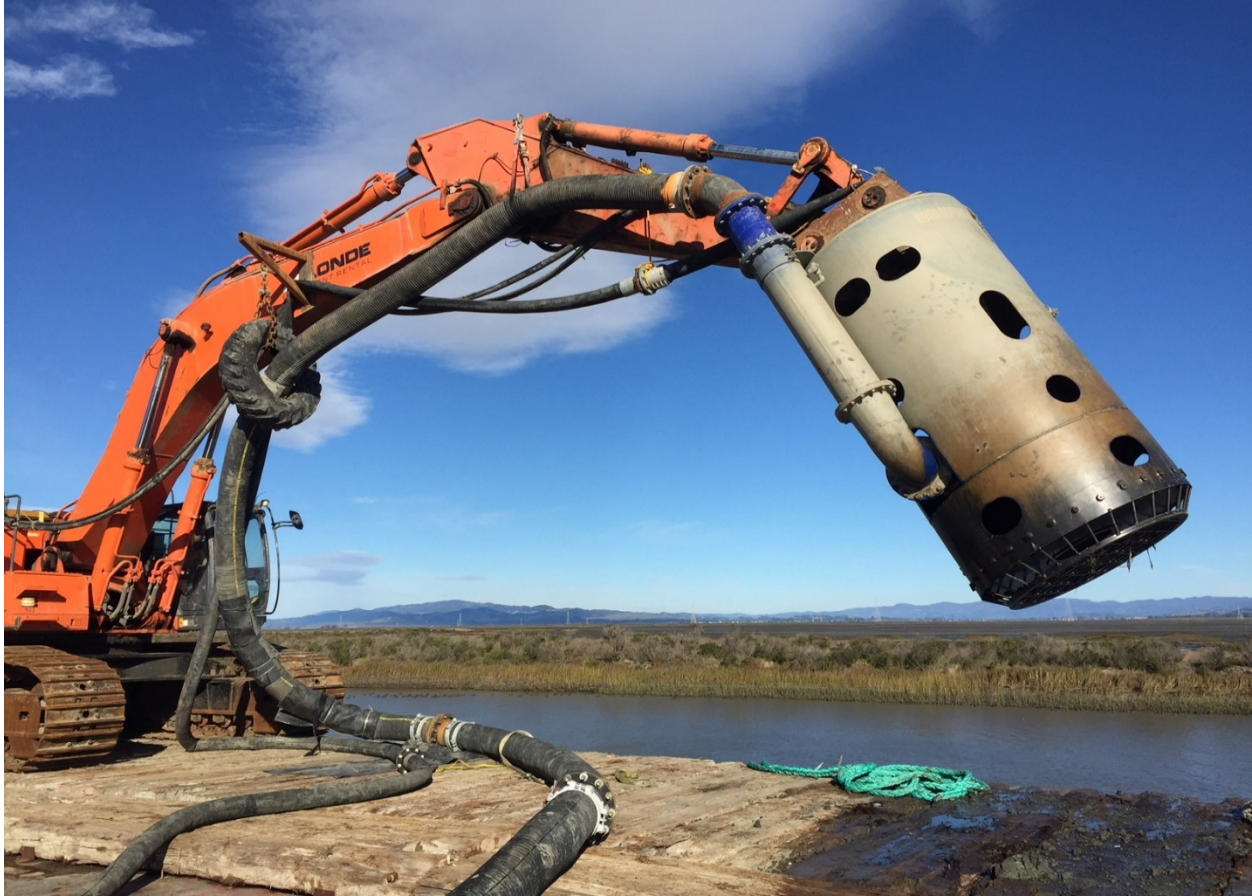
Figure 4 Modified Offloader Currently Offloading Dredged Material at Cullinan Ranch (Dutchman Slough)
