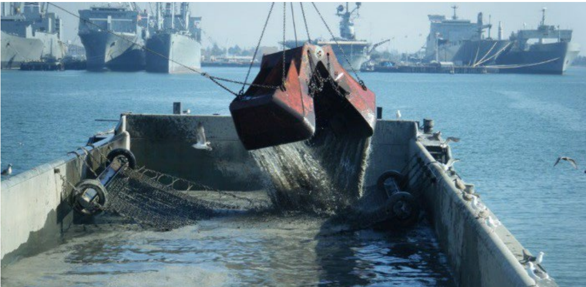
Figure 7 Chain grizzly (California). Photo from DMMP 2015.
