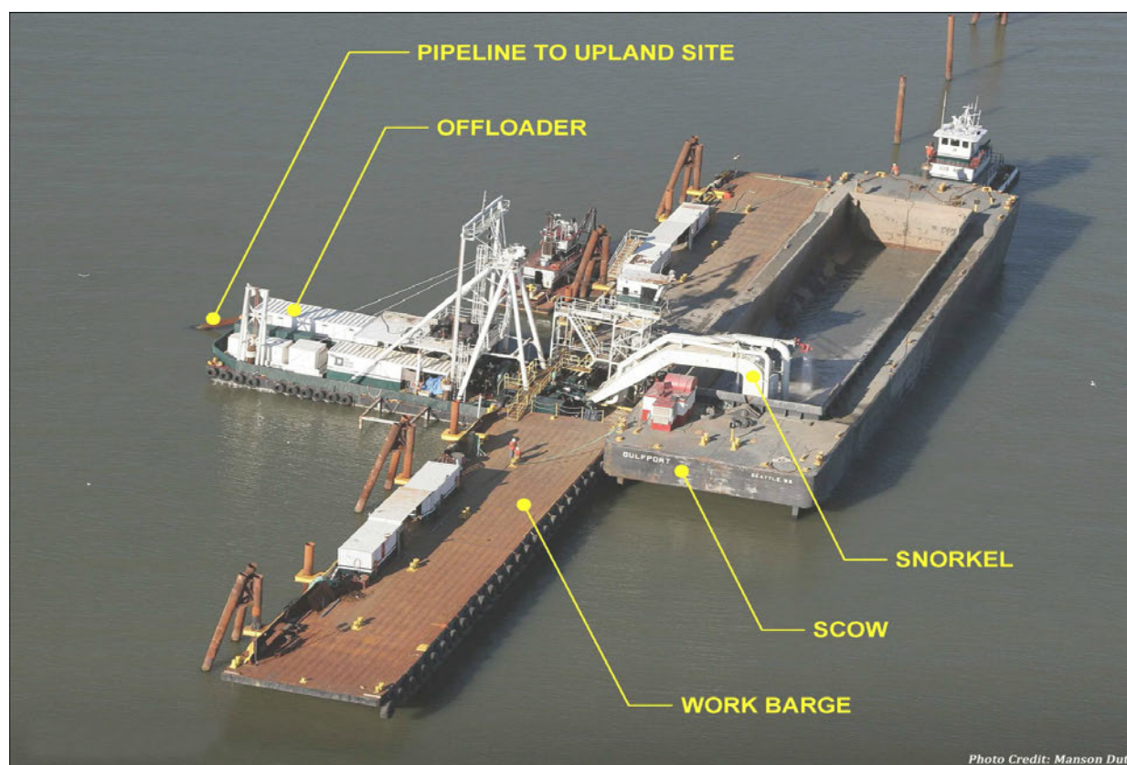
Figure 9 Liberty Offloader during Typical Offloading at Montezuma Wetlands Restoration Project
