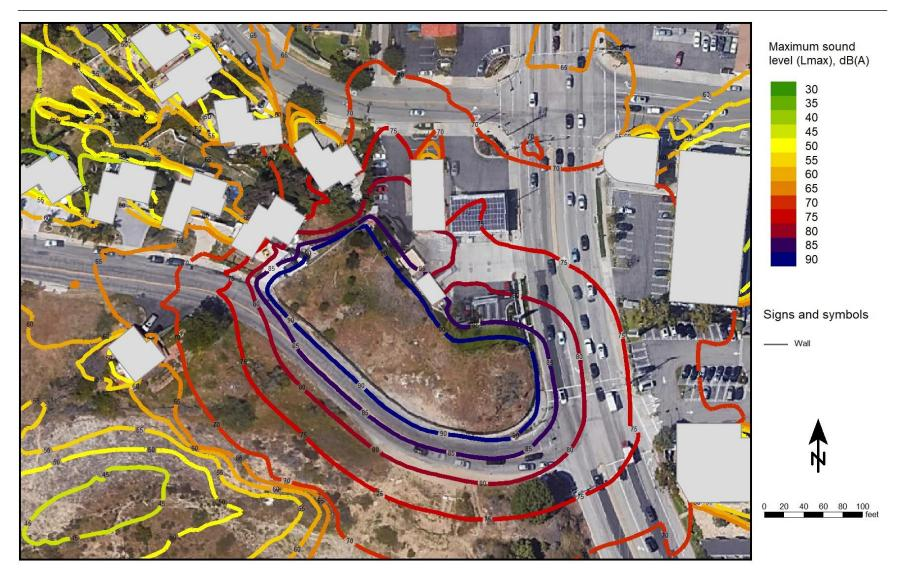
Figure 7 Unmitigated build phase noise contour map
