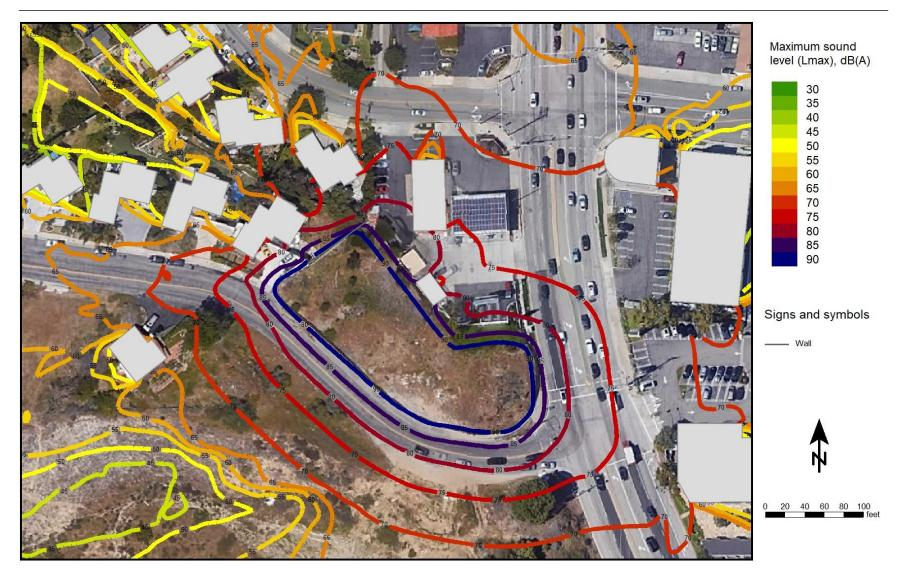
Figure 6 Unmitigated excavation phase noise contour map
