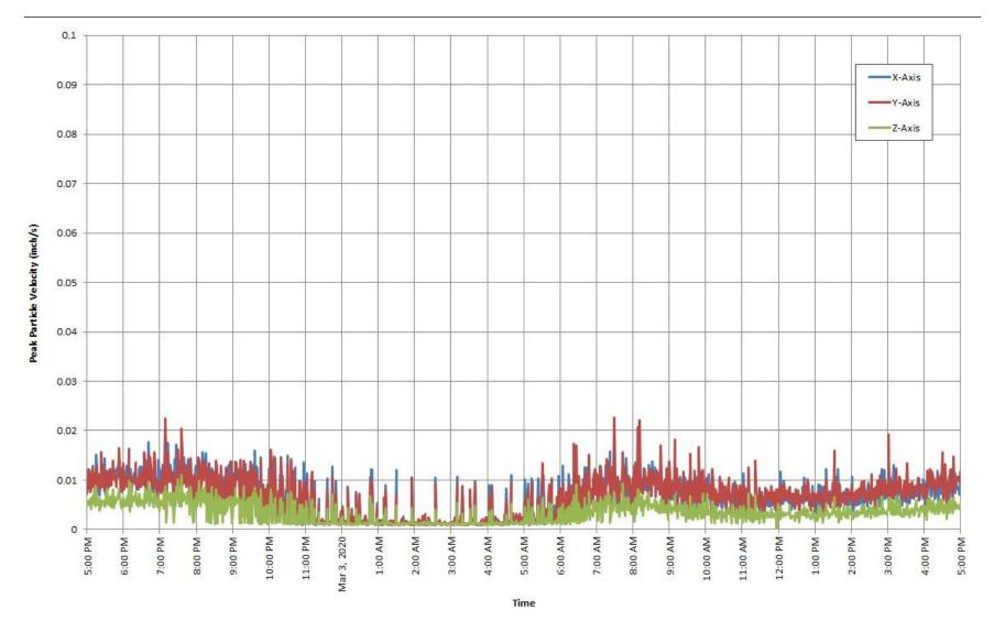
Figure 5 Measured ambient vibration levels
