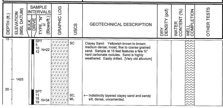
Bottom of boring at 21.5 ft. No groundwater encountered. Boring backfilled with compacted soil cuttings.
