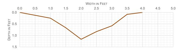
CHART 3. CROSS-SECTION OF DRAINAGE A DOWNSTREAM OF ROAD.
