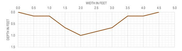
CHART 2. CROSS-SECTION OF DRAINAGE A UPSTREAM OF ROAD.
