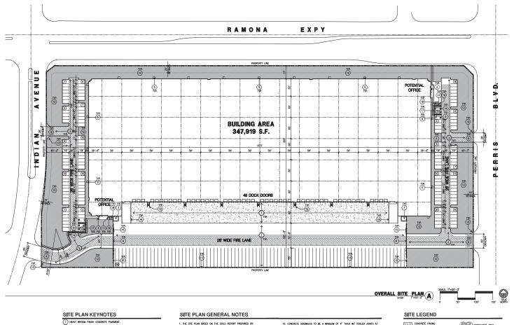
1. THE SITE PLAN BASED ON THE SOILS REPORT PREPARED BY: 2. IF SOILS ARE EXPANSIVE IN NATURE, USE STEEL REINFORCING FOR ALL SITE CONCRETE. 3. ALL DIMENSIONS ARE TO THE FACE OF CONCRETE WALL, FACE OF CONCRETE CURB OR GRID LINE U.N.O.  $\,$ 5 5'-6"X5'-6"X5' THICK CONCRETE EXTERIOR LANDING PAO TYP, AT ALL EXPERIOR MAN DOORS TO LANDSCAPED AREAS. FINISH TO BE NEDIMIN BROOM FINISH.
