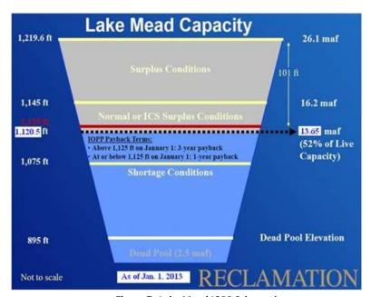
Figure 7. Lake Mead IOPP Schematic
