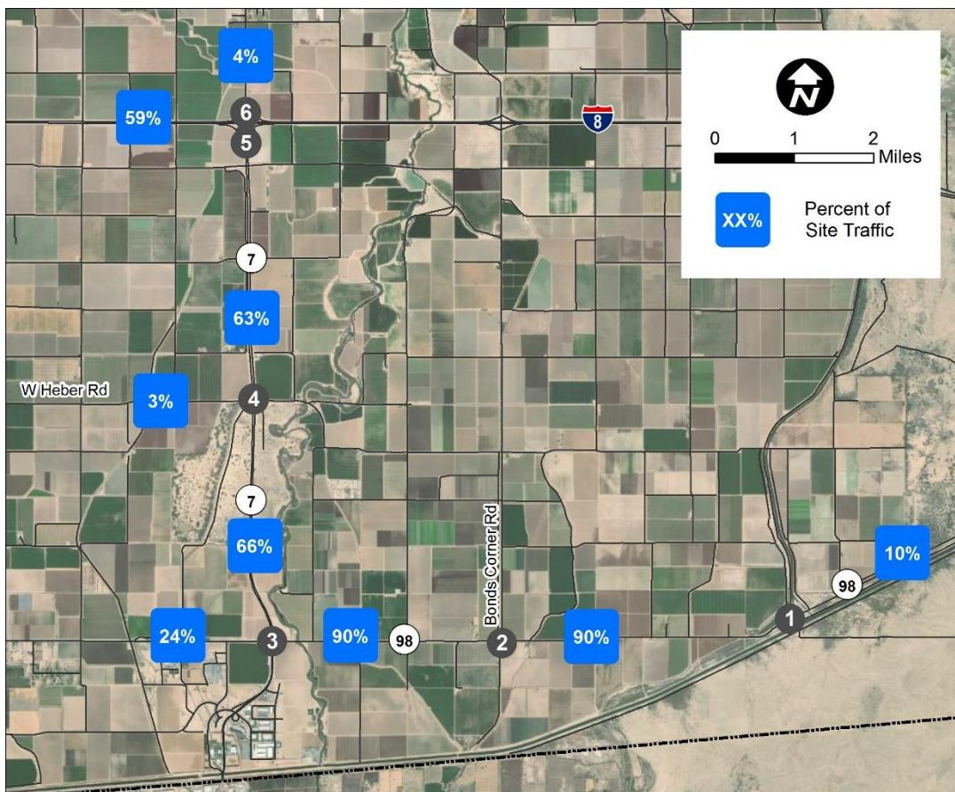
The trip distribution for heavy trucks would require crossing the All America Canal at Gordon Wells Drive. It is estimated that 90% of heavy trucks will travel to the site on eastbound I-8 to the Gordon Wells Drive interchange. The remaining 10% will travel on I-8 westbound. As shown in Table 4.1, only 8 truck trips per day are estimated to use this route.
