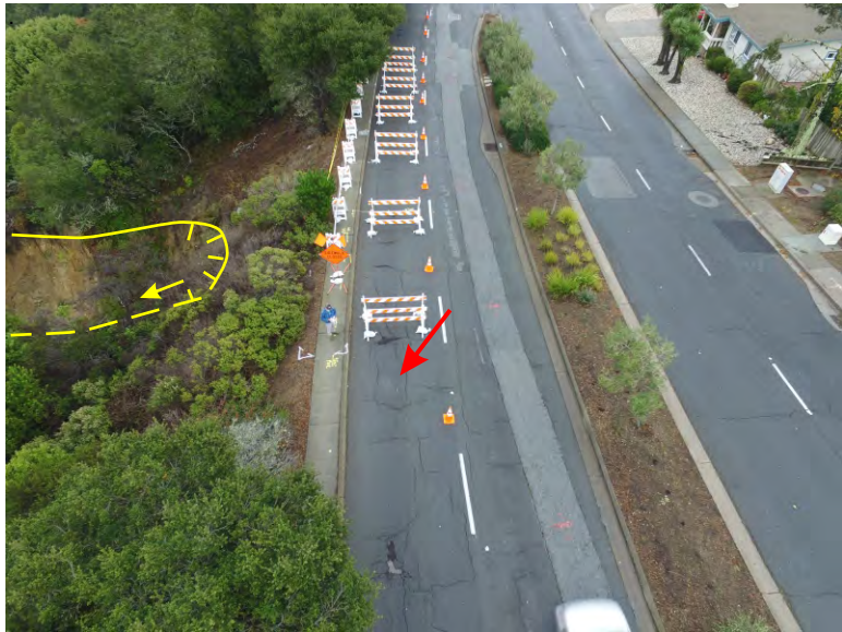
Image 3. East view of headward erosion toward San Bruno Avenue. Arrow points to dilapidated asphalt roadway.
