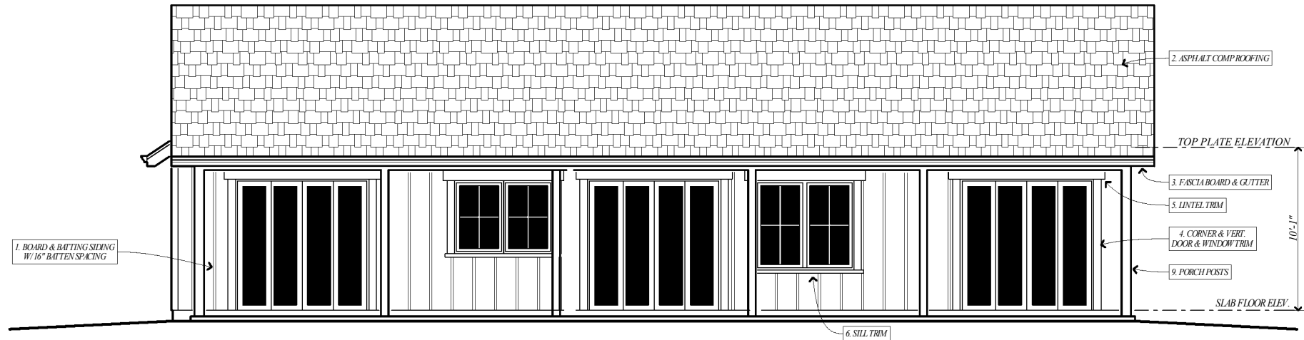
REAR / EAST SIDE EXTERIOR ELEVATION SCALE: 1/4" = 1'-0"
