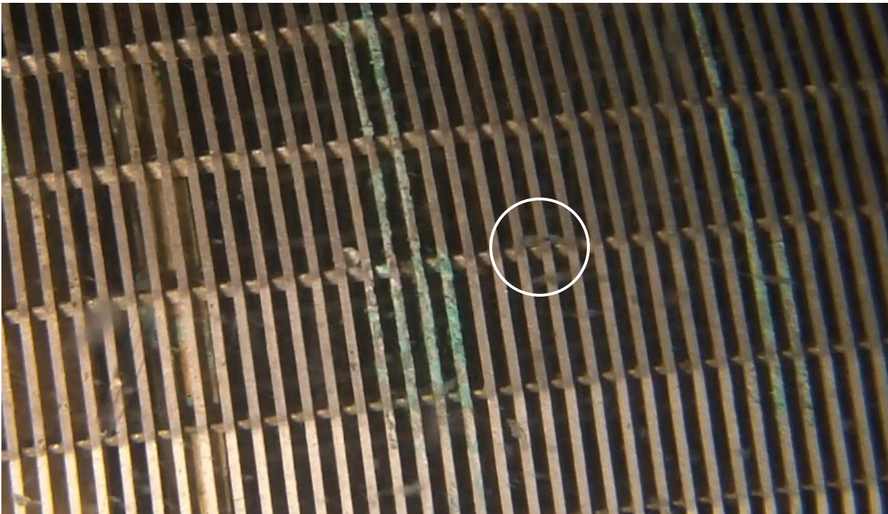
Figure 2.1 Picture of fish larvae swimming near a wedge-wire intake screen with the pump operating
