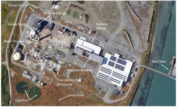
Image 2-2 Project Existing Site Conditions for the Terrestrial Development and Location of the Water Intake (Sea Chest) on the RMT II Dock
