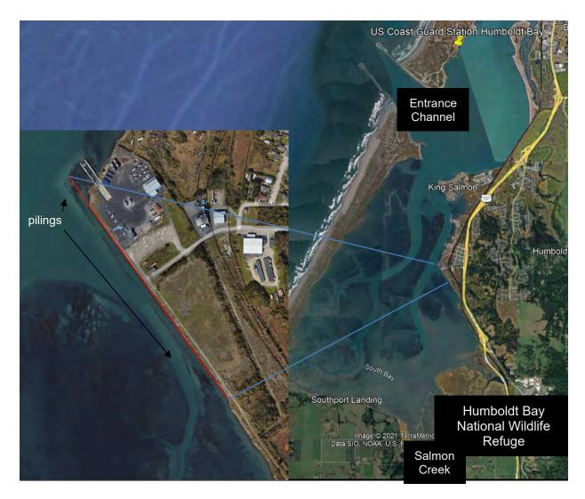
**Figure 1**. Map of South Bay area of Humboldt Bay with inset showing detail of pilings from the abandoned Kramer Docks. The red line in the inset is 560 m (0.35 mi) long and shows the extent of the pilings along the shoreline.
