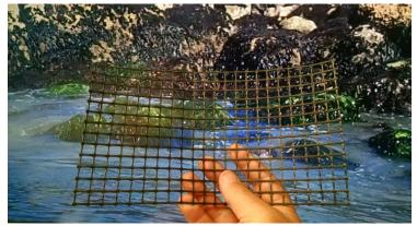
HDPE grid to be used to attach surfgrass to breakwater rock with marine epoxy in small test plots. The plots will be established along differing portions of the breakwater in clusters to evaluate longterm survival and growth of plants under different circumstances and the capacity to conduct such transplants at a scale and with the performance certainty necessary to serve as compensatory mitigation.
