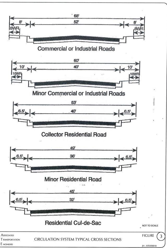
The desirable goal for every roadway in the Circulation Element is that it carries the existing and future traffic volumes of traffic at the desired level of service. To achieve this requirement variation in design is expected depending on factors such as the capacity needs and the adjacent land uses. Such variations will involve on-street parking, sidewalks, pathways, bicycle lanes, bike paths, median landscaping.
