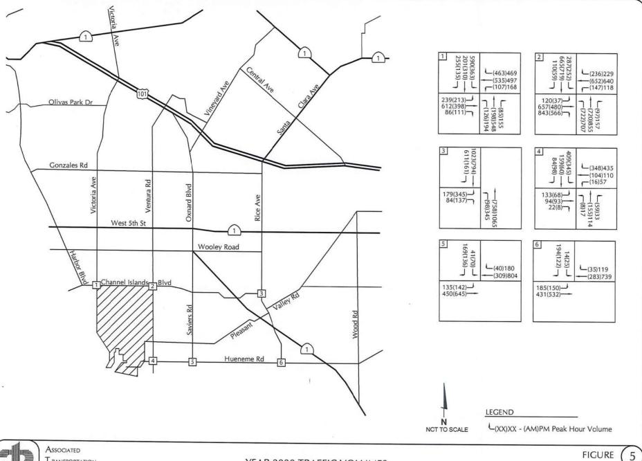
Year 2020 levels of service were calculated for the study-area intersections using the Intersection Capacity Utilization (ICU) methodology for signalized intersections as required by the City of Port Hueneme. Worksheets illustrating the level of service calculations are contained in the Technical Appendix for reference. Table 1 lists the level of service for the study-area intersections during the AM and PM peak hour periods.
