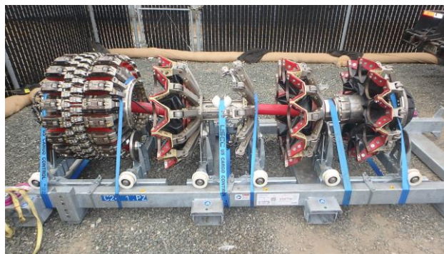
Figure 30 – Electro Magnetic Acoustic Transducer (EMAT) Tool Before an Inspection on L-210C
