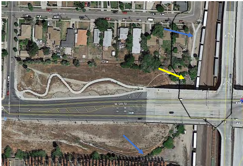
April 2014 – After construction of concrete ditch within buffer (northern blue arrow) to direct flows from road and railroad track under I-215 off-site through concrete ditch (southern blue arrow). Riprap basin remains (yellow arrow).
