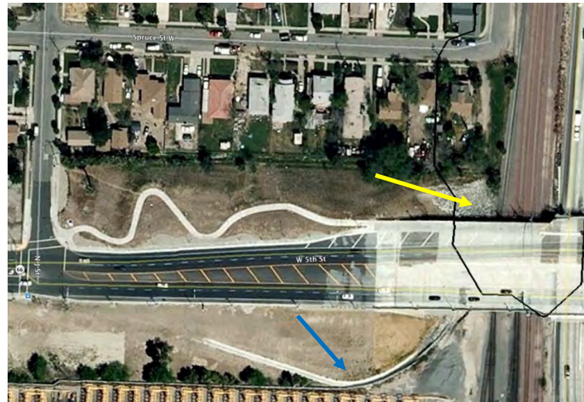
June 2009 – After placement of riprap basin (yellow arrow) and construction of concrete ditch off-site (blue arrow), routing flows from buffer.
