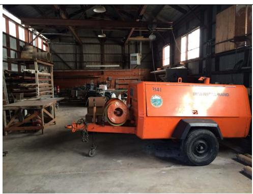
Photo 6: Twenty-four-gallon diesel-powered mobile air compressor located in the carpentry room of the building located along the southern Site boundary.
