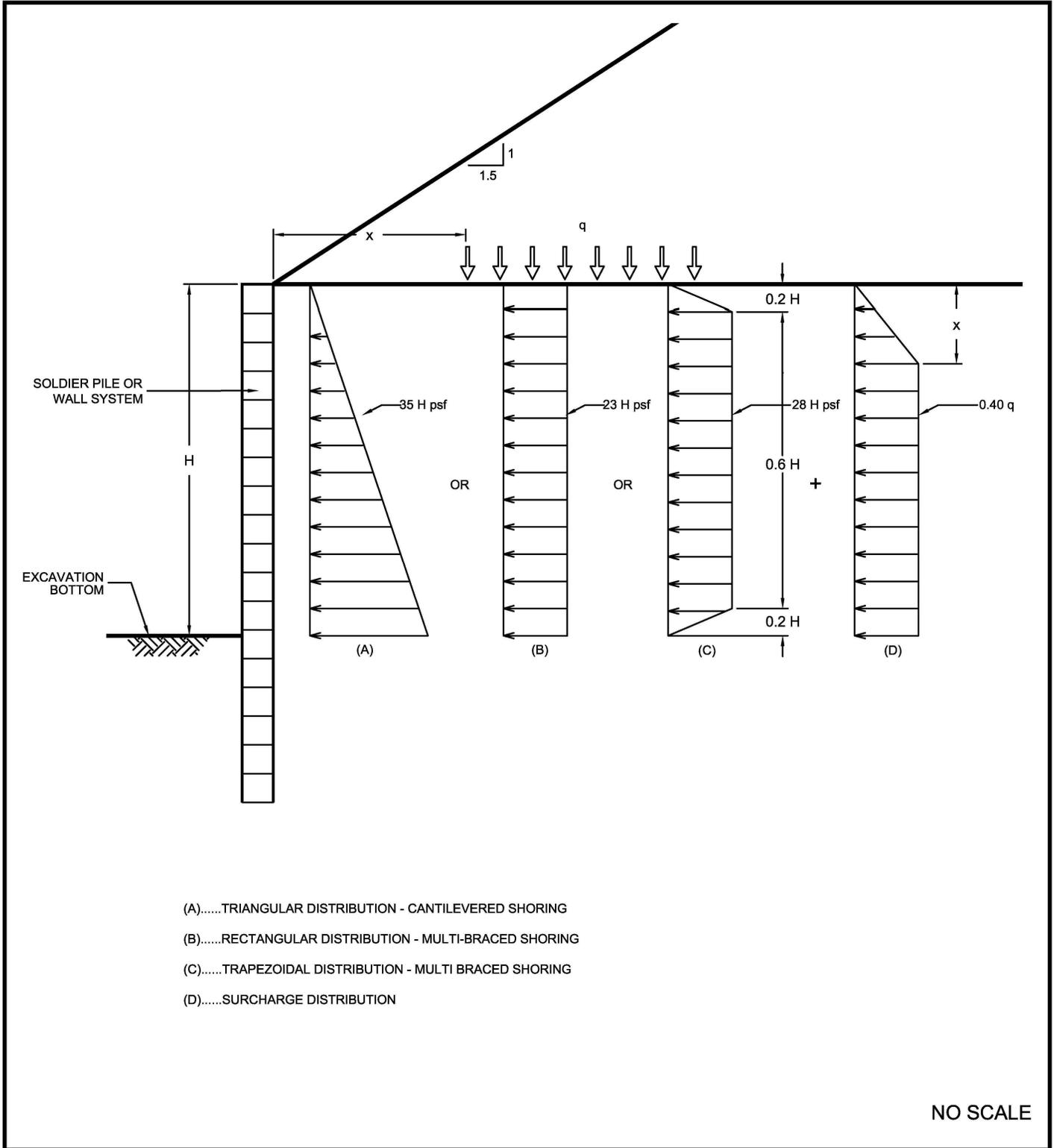
LATERAL ACTIVE PRESSURES FOR VERTICAL EXCAVATIONS
