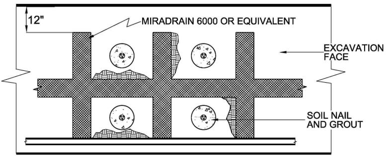
DRAINAGE PANELS PER SOIL NAIL WALL ENGINEER
