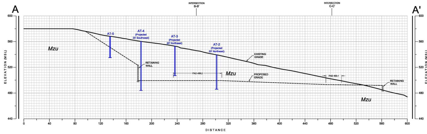
**GEOLOGIC CROSS-SECTION A-A'**
