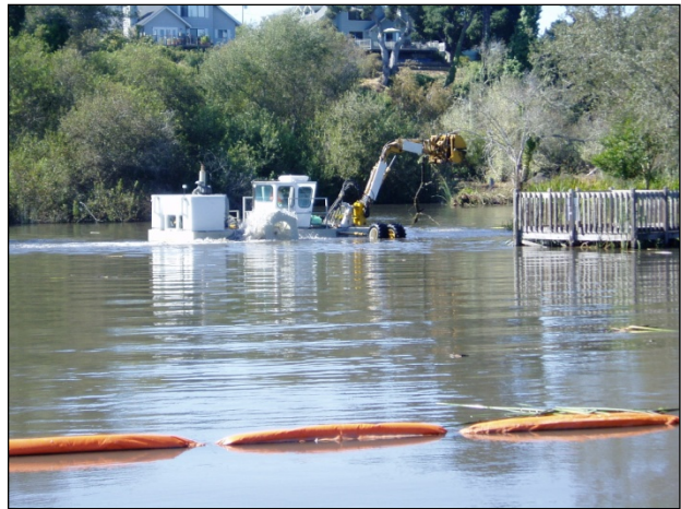
LEFT: Aquamog with clamshell and weed harvester in operation during tule removal. RIGHT: Aquamog in upper lagoon.
