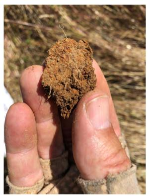
Photo 7. Redox features from data point 1A in feature #16.
