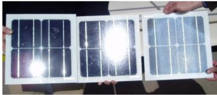
Figure 2-2: Example of Specular and Diffuse Reflections
