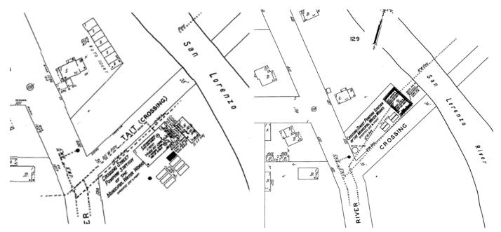
Figure 9. Comparison of the 1928 Sanborn Map (left) showing the old Crossing Street Pumping Plant and the 1928-1950 Sanborn Map showing the new facility completed in 1929 in approximately 1945 (right) (Sanborn Map Company 1928: 103, 1928-1950: 103).
