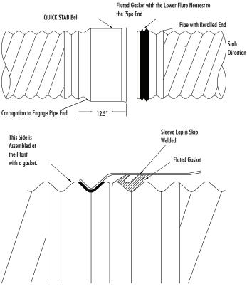
The Bell and Spigot joint is available on ULTRA FLO and  $2-2/3'' \times 1/2'''$  corrugation in 15" through 60" diameter.
