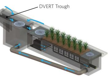
them over to a connecting pipe exiting out the wall of the inlet and leading to the MWS Linear. The DVERT is perfect for retrofit and green street applications that allow the system to be installed anywhere space is available.
