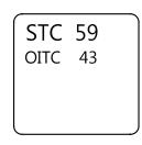
Mass-air-mass resonant frequency = =54 Hz Panel Size = 8.9 ft x 13.1 ft Partition surface mass = 12.4 lb/ft2
