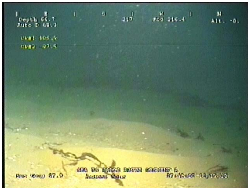
Figure 3: Coarse sand substrate in < 30 m water depth offshore Southern California. Drift kelp and ornate tube worms ( D. ornata ) along the SEA-US cable route.
