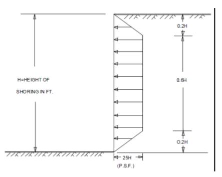
The recommended earth pressure provided above is preliminary value. The design earth pressure should be estimated based on the depth of the excavation, type of the retaining structure and soil properties.
