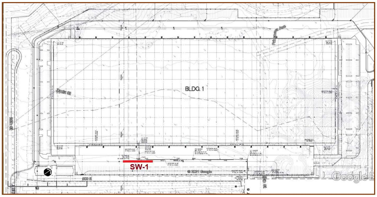
BASE MAP: Site Plan prepared by Thienes Engineering, Inc. (partial copy, Conceptual Utility Plan, Sheet 7 of 13); Seismic shear-wave traverse SW-1 shown as red line.
