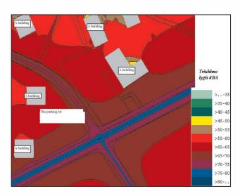
Fig 8. Results of the simulation of noise dispersion at the parking lot on Ateities street
