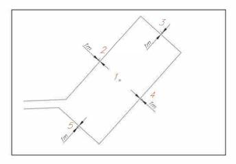
Fig 1. Layout of noise measuring spots at the parking lot on Architektų street: 1 - in the centre of the lot, 2-5 - ata distance of 1 m from the lot
