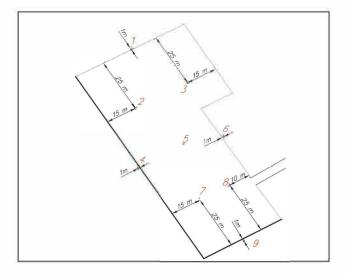
**Fig 3.** Layout of noise measuring spots at the parking lot on Ateities street: 5 - in the centre of the lot, 2, 3, 7, 8 - i within the lot, 1, 4, 6, 9 - at a distance of 1 m from the lot
