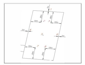
**Fig 5.** Layout of noise measuring spots at the guarded parking lot on Č. Sugihara street: 5 - in the centre of the lot; 2, 3, 7, 8 - within the lot, 1, 4, 6 - at a distance of 1 metre from the area of the lot
