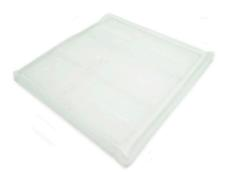
Paint Filter Pad, Polyester media with ECXL style. The media is multilayered, with finer fiber structures downstream in order to enhance depth loading capacity. The multiple layers will avoid face loading as it captures overspray paint with a downstream tackifier.
