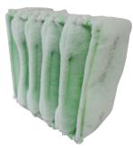
The recommended 3-stage system consists of a prefilter pad, a 2 pocket filter bag, followed by the EPA Method 319 approved 5 pocket bag filter. The 5 pocket bag filter is self sealing and exceeds the testing requirements with or without the pre-filter pad and two pocket filter bag. The media construction is multi-layered with the downstream layer consisting of a high efficiency synthetic media.
