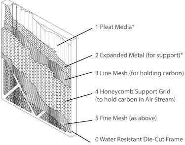
\*NOTE: for 1" version a poly pad and no expanded metal replace the pleat media
