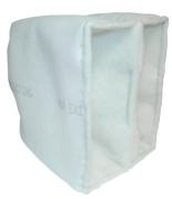
The recommended 2-stage system consists of a prefilter paint arrestor pad followed by a two pocket bag filter. This two pocket bag filter exceeds the approved EPA Method 319 testing requirements with or without the prefilter pad. The 2-pocket filter is self-sealing and has self supporting pockets. The Media construction is a multi-layered gradient density structure to maximize paint collection and retention.
