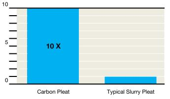
\*Amount of gas or odor removed at 50% break through given 880 PPM of Toluene @ 40 (media velocity)
