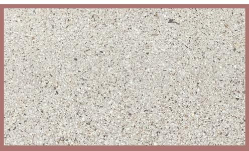
Type 1L concrete with etched finish
