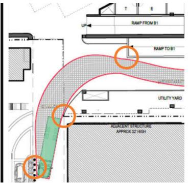
FIGURE 3: LEFT-TURN AT PROPOSED 90-DEGREE BEND IN ALLEY - SU-40 TRUCK
