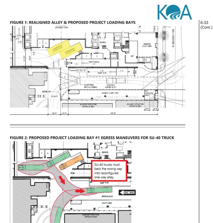
The maneuvers shown in Figure 2 indicate that an SU-40 truck parked in Loading Bay #1 would have to back up eastbound onto the proposed realigned westbound-only alley segment. This contra-flow maneuver could present a safety hazard for motorists turning onto the realigned alley from North Beverly Drive. This maneuvering would conflict with not only automobile traffic generated by the Project, but also
