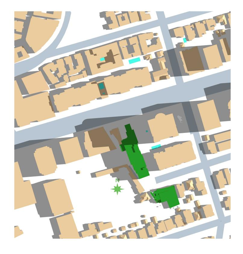
Summer Solstice Shading Diagram 8 a.m.
