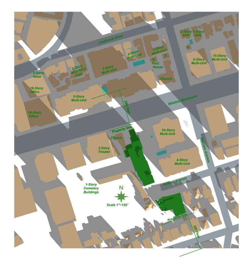
Winter Solstice Shading Diagram 9 a.m.
