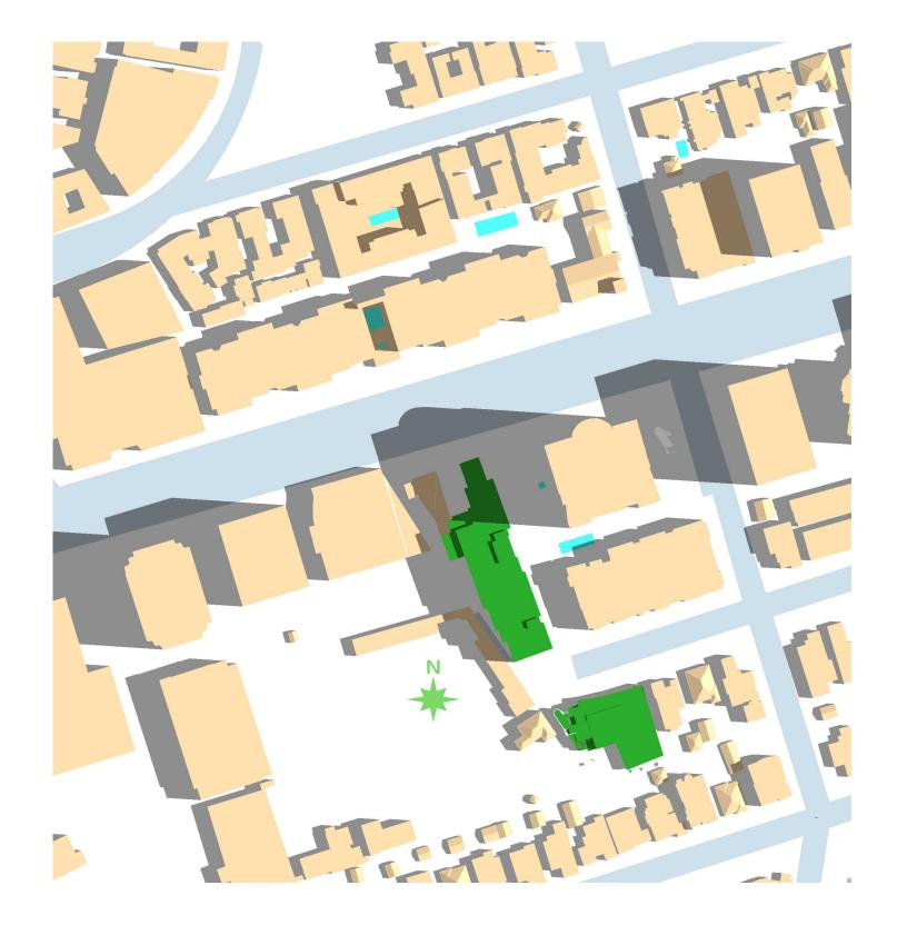
Summer Solstice Shading Diagram 9 a.m.
