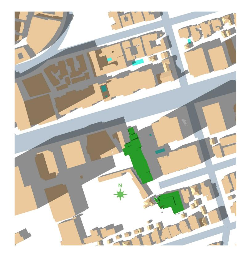
Vernal/Autumnal Equinox Shading Diagram 3 p.m.
