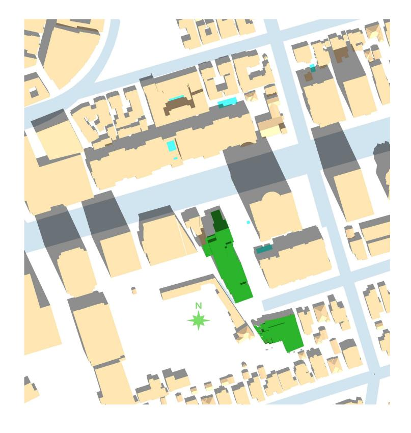
Vernal/Autumnal Equinox Shading Diagram 11 a.m.
