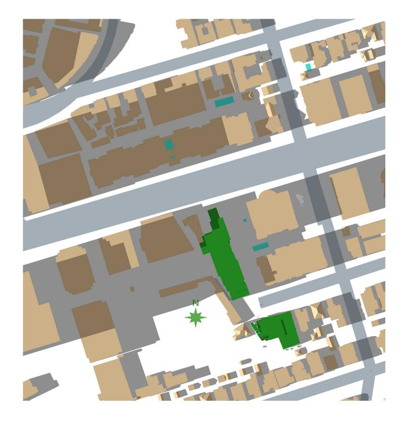
Vernal/Autumnal Equinox Shading Diagram 4 p.m.
