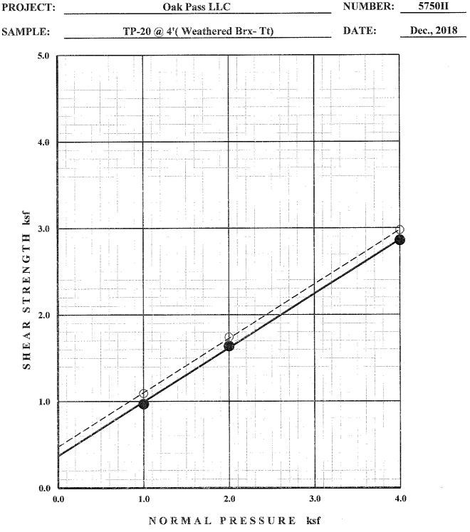
STRAIN RATE -0.005 in/min SAMPLE SATURATION - 24 hrs Final moisture content =
