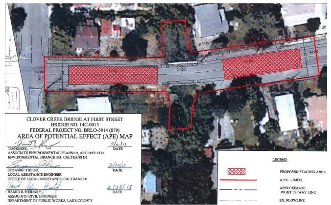
Figure 1. Proposed staging area and road closure during construction.
