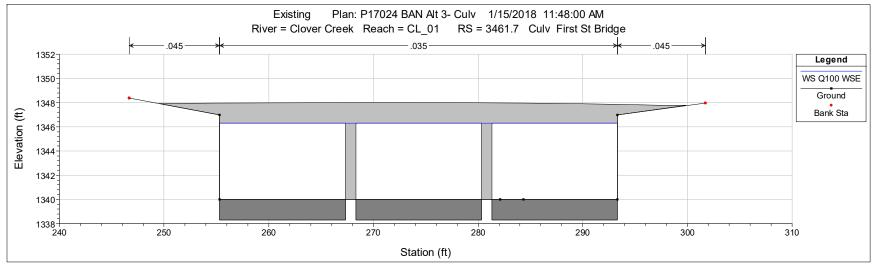
Figure 12. Upstream Face of Proposed Culvert, Looking Downstream (South)
