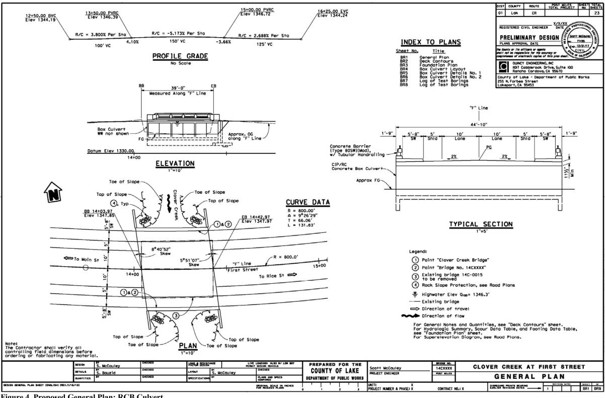
Figure 4. Proposed General Plan: RCB Culvert
