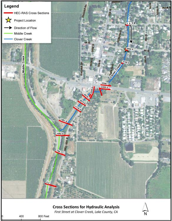
**Figure 9. Cross Section Locations**
