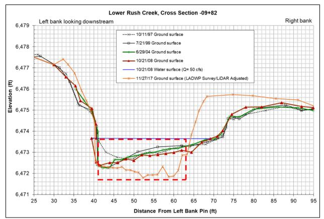
Figure 1. Example Historical Cross Section Survey Comparison - Rush Creek XS -09+82
