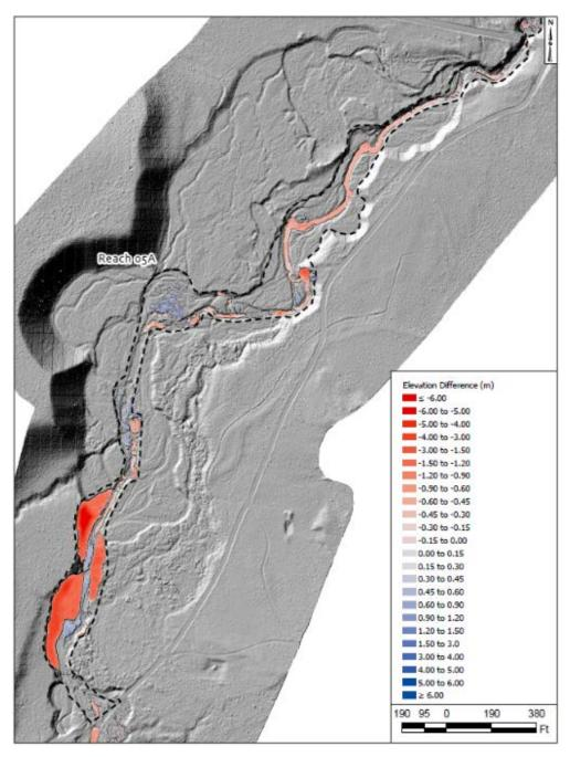
Figure 3. Example Geomorphic Change Detection Map (from Pre- and Post-Peak 2017) – Rush Creek Reach 5A (Upper Portion)
