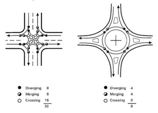
The number of conflicting points for the roundabout and signal alternative can be understood from the insert above. The analysis above illustrates the advantages that the roundabout alternative provides by significantly reducing the number of conflict points between vehicles and further justifies the higher CMF values as the exposure to risk is significantly reduced at roundabout intersections.
