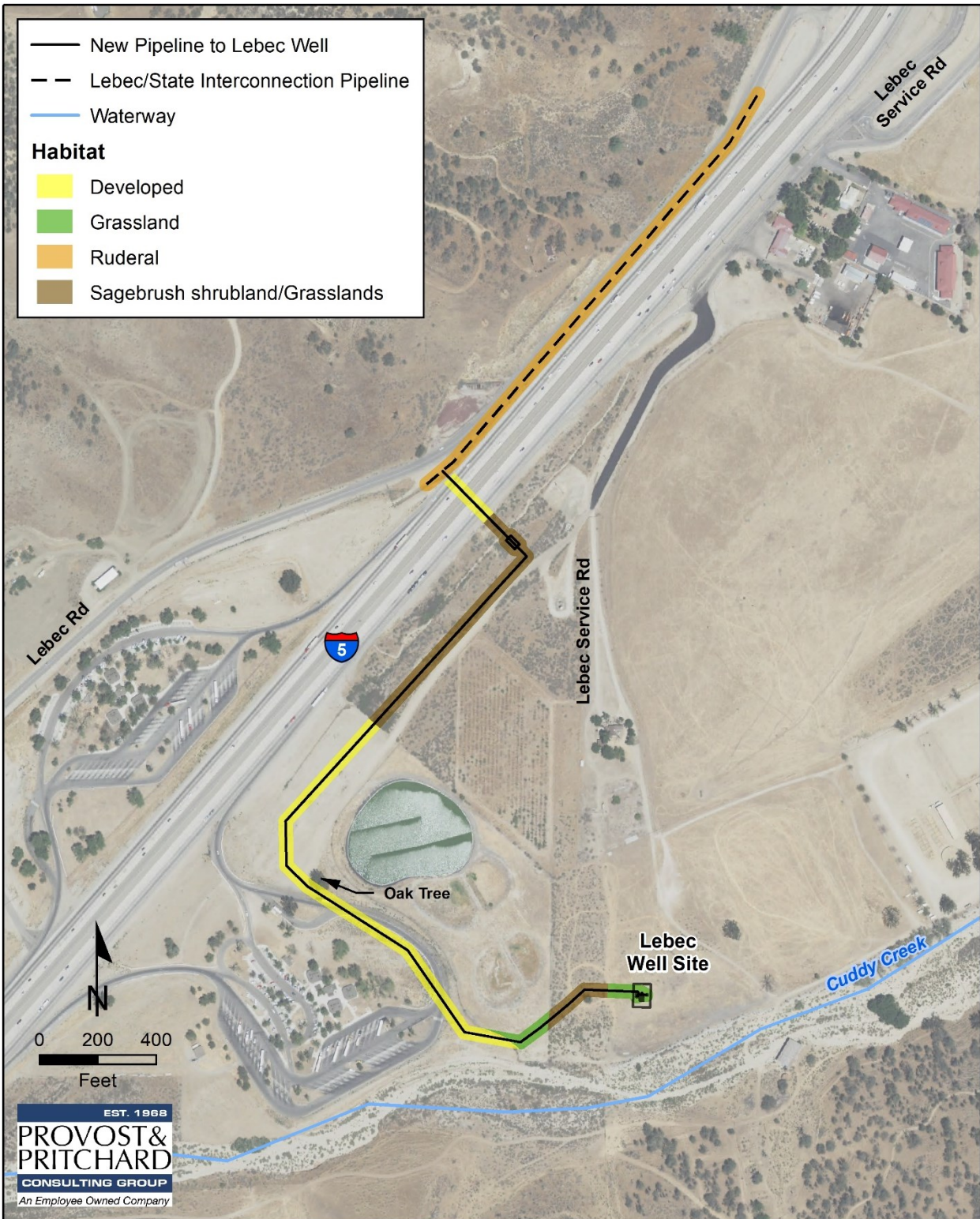
Figure 4. Detail of New Pipeline to Lebec Well 04 & Lebec/State Interconnection Pipeline
