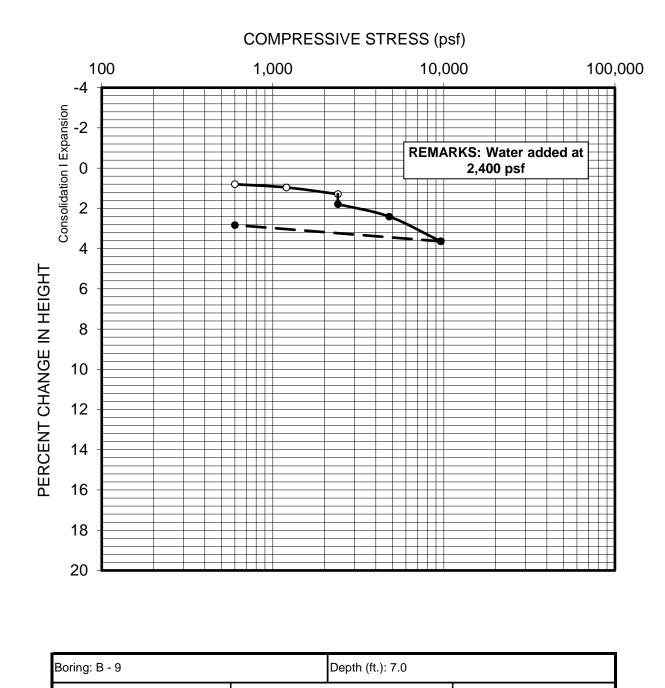
Dry Density (pcf): 120.0Saturation (%): 39.3Moisture (%): 5.9Sample Description: Silty sand (SM), cemented. [Very old alluvium]
