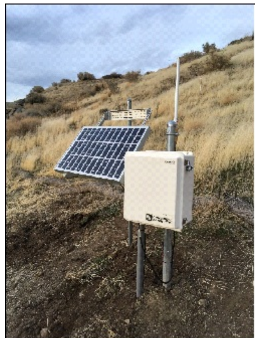
Figure C.4. Automated Data Acquisition System (ADAS) similar to the systems to be installed in Montecito.
