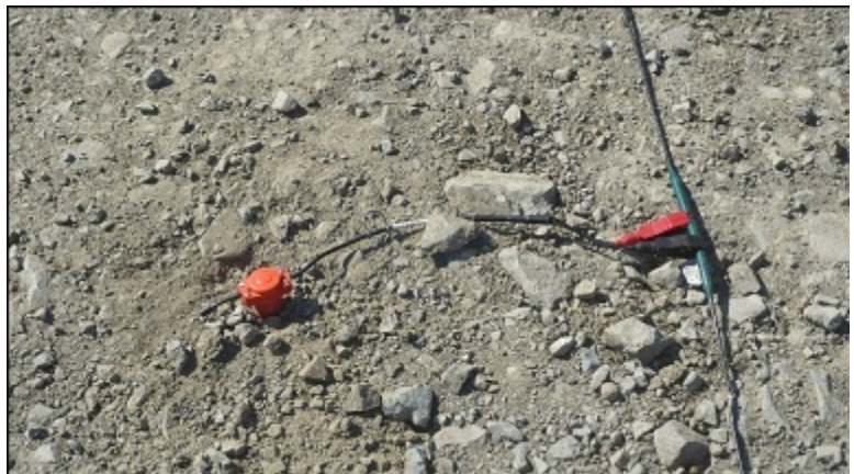
Figure C.1. Geophone installed in subsurface.
