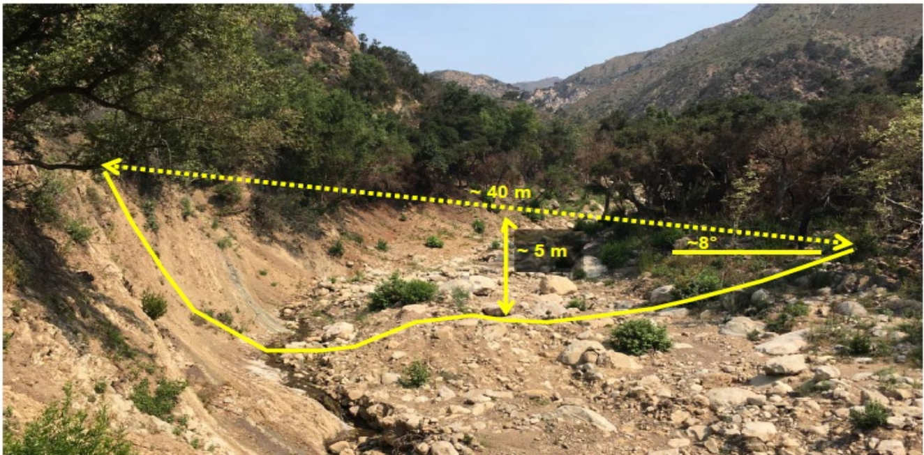
Figure 8. Superelevation of January 2018 flow indicated by mud lines in Cold Spring Canyon approximately 300 m upstream from the development interface. BGC photo, July 2018, looking north.
