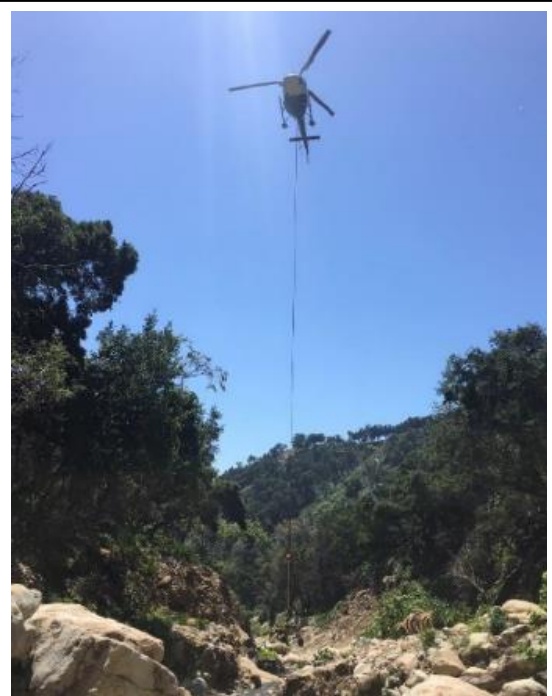
Photograph 6. Heavy construction equipment (e.g., Spyder excavator or 10-ton class excavator and conveyor belt system) would be airlifted to via helicopter for major maintenance activities.
