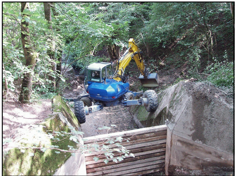
Figure 14. The Kaiser Spyder S2 Walking Excavator. It is specialized, low-environmental-impact drilling equipment from Access Limited. The machine recently was used to install anchors for debris nets Camarillo, California. Note that machine is supported on sides of channel and does not disturb the channel itself. Pictured here with an excavator bucket. The machine can be configured with a drill for anchor installation or a bucket for net clean-out.
