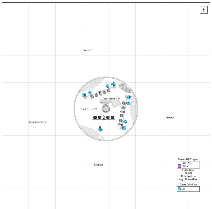
Note that the areas shown in purple are where AT&T antennas contribute more than 5% of the FCC's general exposure RF limit. These do not overlap any areas in front of other carrier antennas exceeding the FCC's general exposure RF limit because there are no other carriers as shown in Figure 1. Under FCC regulations, AT&T is therefore not responsible for predicted exceedances of another carrier's antennas.
