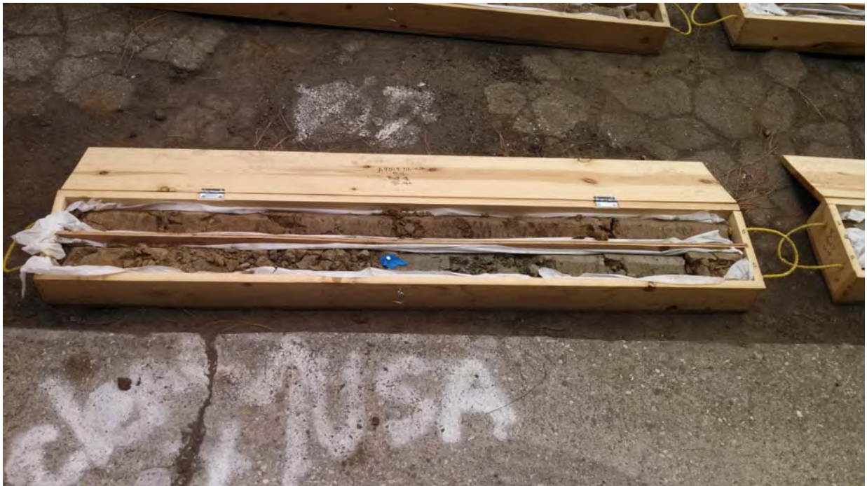
Photo 17: Core sample boring B4-A at 30 to 40 feet
