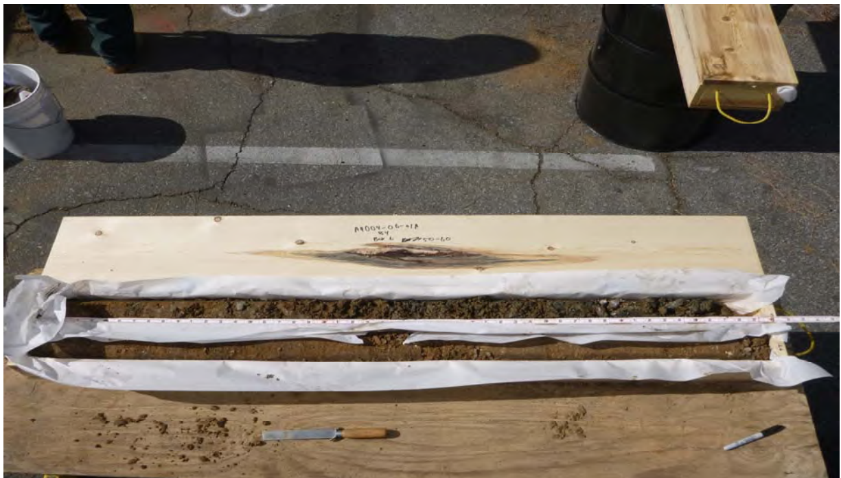
Photo 18: Core sample boring B4-A at 50 to 60 feet
