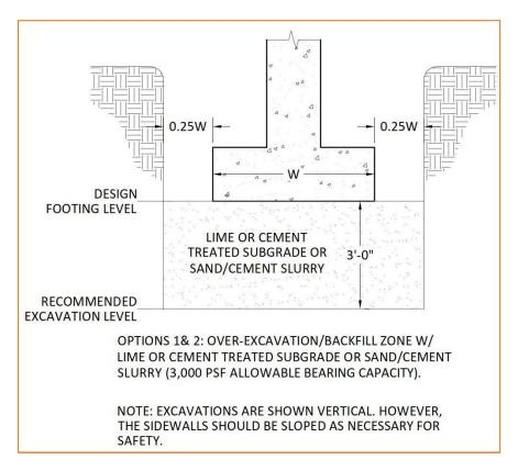
Over-excavation for structural fill placement below footings should be conducted as shown below. The over-excavation should be backfilled up to the footing base elevation, with engineered fill placed, as recommended in the **Earthwork** section.
