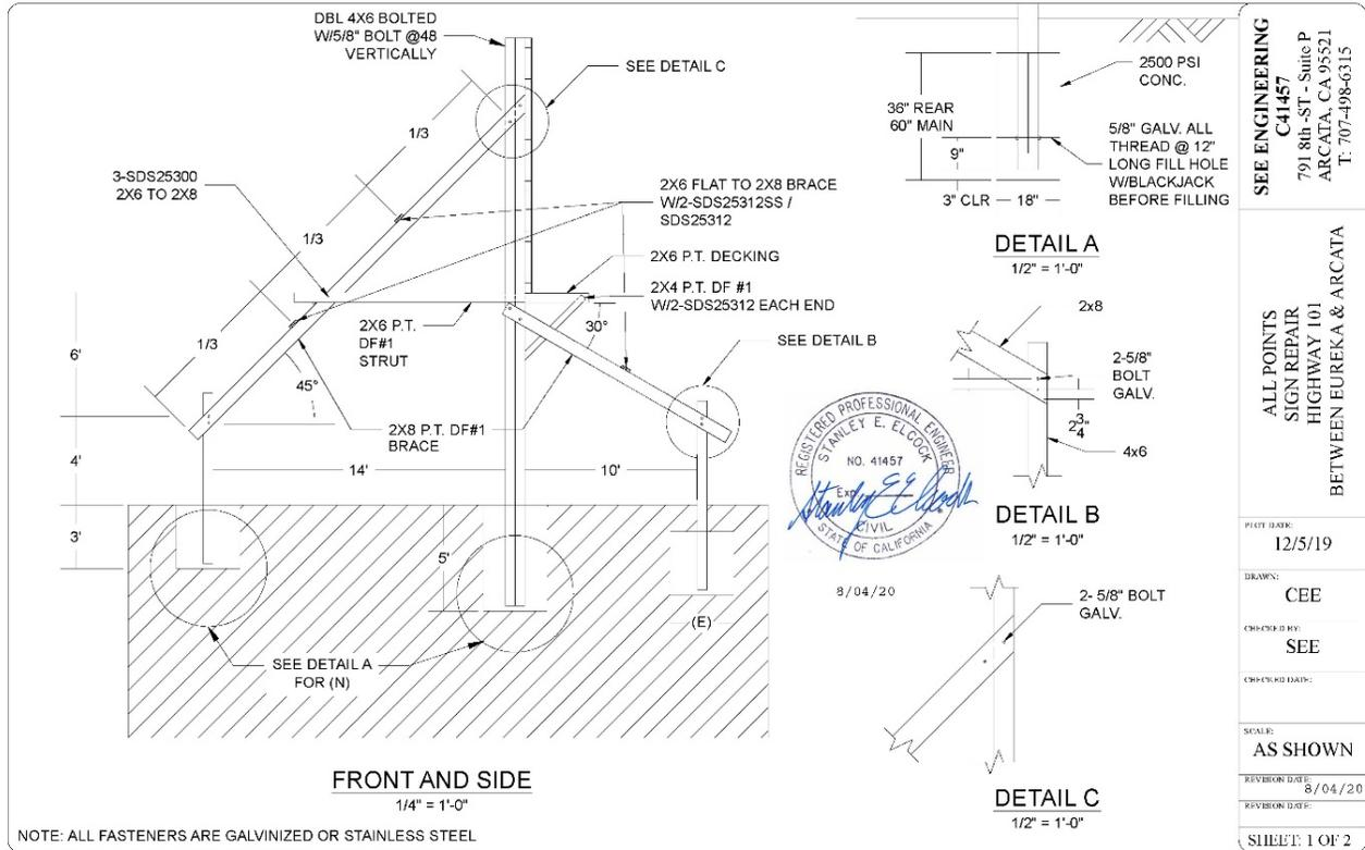
Figure 20: Engineered Plans for Sign Repair – Profile View showing footing & bracing detail
