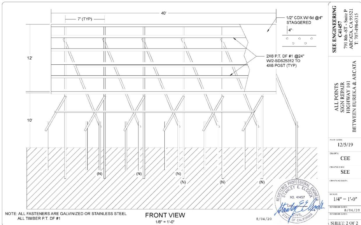
Figure 19: Engineered Plans for Sign Repair – Front View
