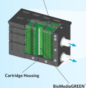
Vertical Underdrain Manifold
