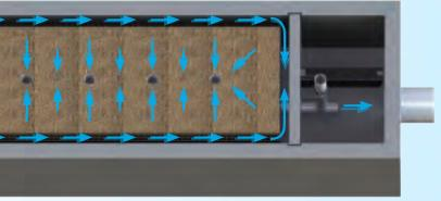
2x to 3x more surface area than traditional downward flow bioretention systems.
