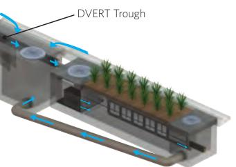
to a connecting pipe exiting out the wall of the inlet and leading to the MWS Linear. The DVERT is perfect for retrofit and green street applications that allow the Modular Wetlands<sup>®</sup> to be installed anywhere space is available.
