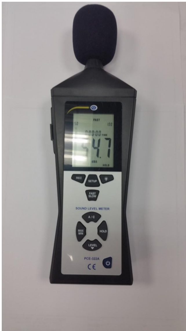
Figure 3: PCE-322A noise meter used in study
