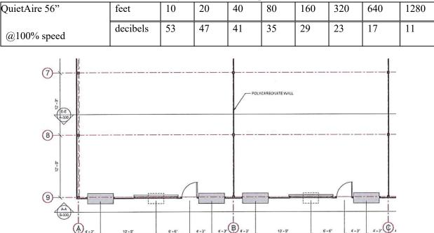
Table 14. Greenhouse exhaust fan dBA analysis -one (1) fan as point source
