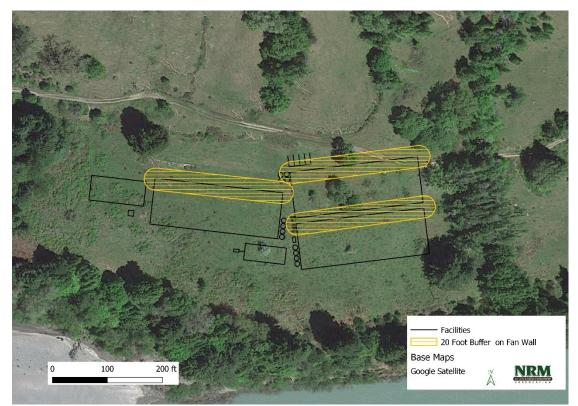
Figure 29. 20-foot buffer around fan walls: Facilities #1 through #3
