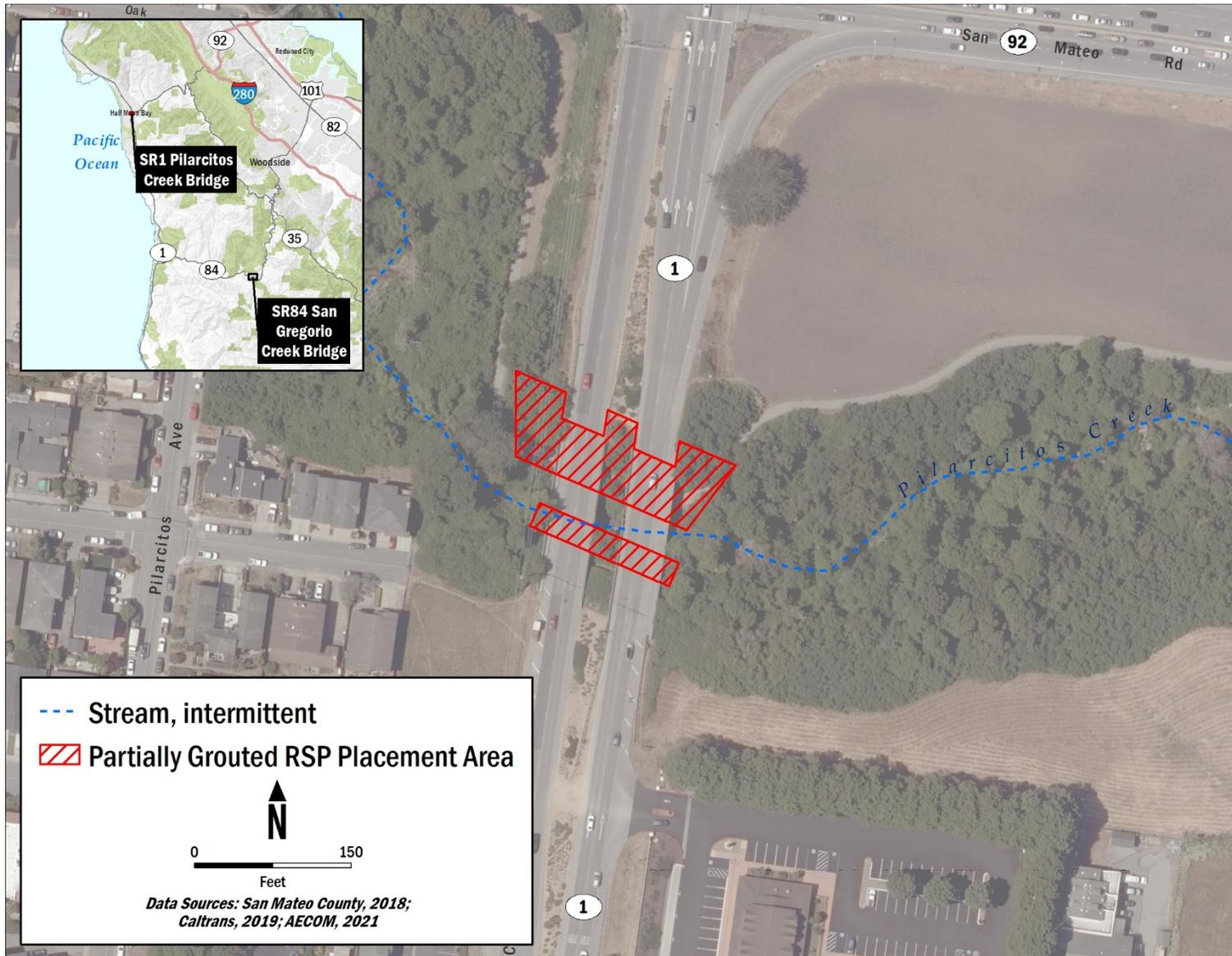
Figure 7 State Route 1 at Pilarcitos Creek Bridges Project Proposed Partially Grouted RSP Placement
