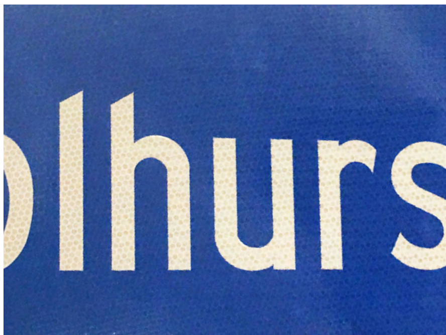
Figure 116. Retroreflective substrates, colored film, and clear anti-graffiti film layer on top of aluminum to create the graphic of a sign. Source: OLIN, 2019.
