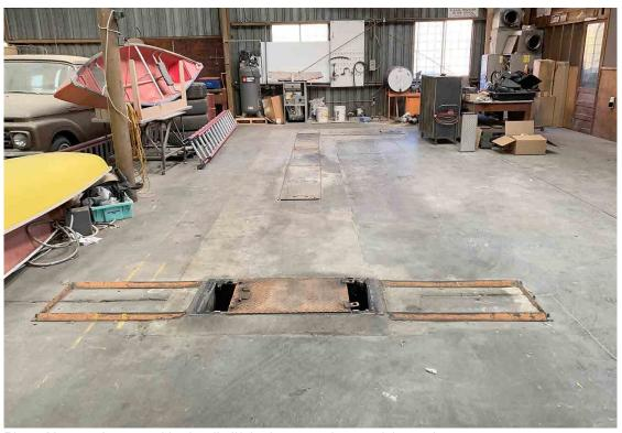
Photo No. 22 In-ground hydraulic lift in the central area of the maintenance garage.
