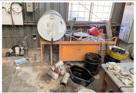
Photo No. 21 New and used motor oil containers, used oil filters, and minor oil spills in the work area in the eastern portion of the maintenance garage.
