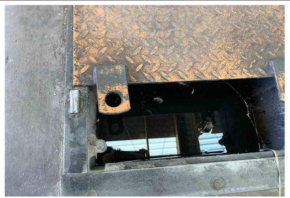
Photo No. 23 Front section of the hydraulic lift filled with an oil-like fluid.
